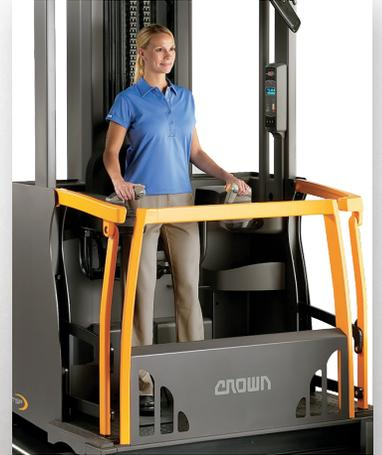
**Standing Tasks** are efficiently accomplished with a seat that folds up and controls that adjust to the operator height.
